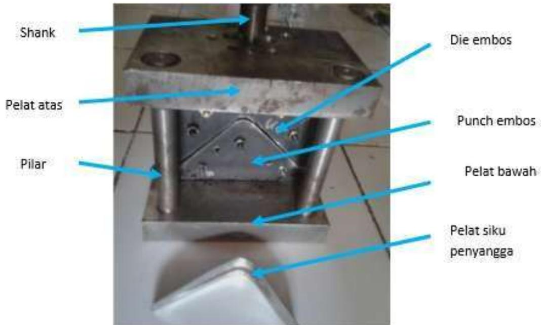
**Gambar 5. Alat bantu compound tool**
