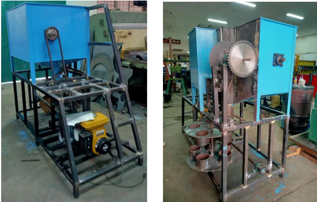
Gambar 3 Purwarupa Mesin Press Baglog Jamur
