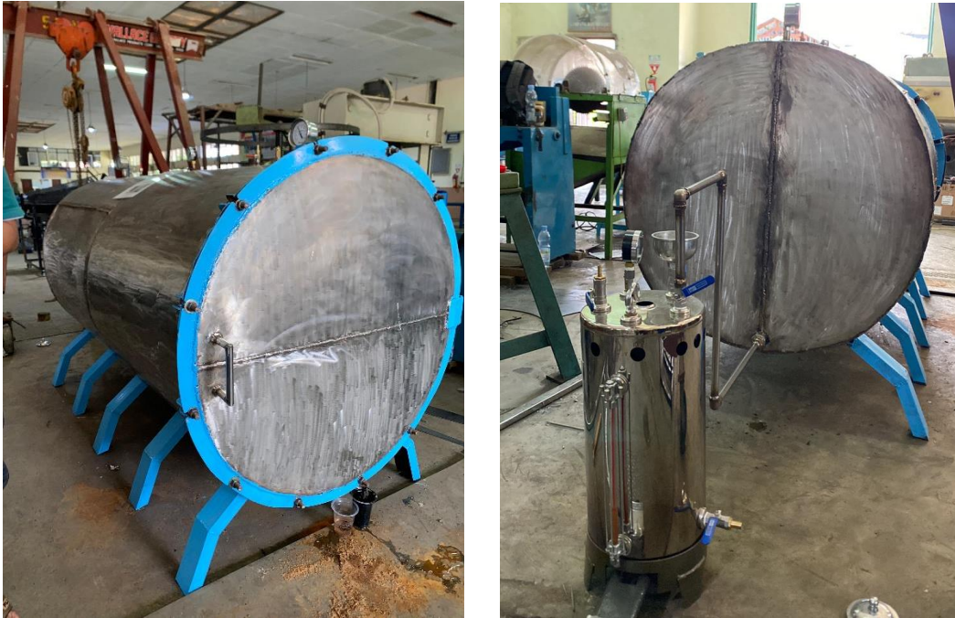
Gambar 1 Purwarupa Mesin Steamer baglog Baglog
