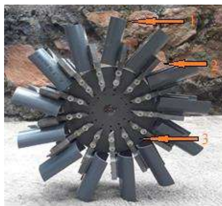
Gambar 4. 1 Runner Turbin Pelton: (1) sudu/mangkok turbin; (2) kaki dan penahan sudu; (3) piringan/cakram.
