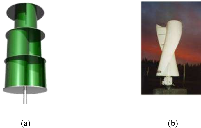
Gambar 2. Bentuk turbin Savonius : (a) Two-bladed-multi stage Savonius , (b) Twisted blade Savonius
