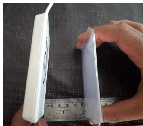
Picture 4.1 Testing the distance of the read card by the reader
